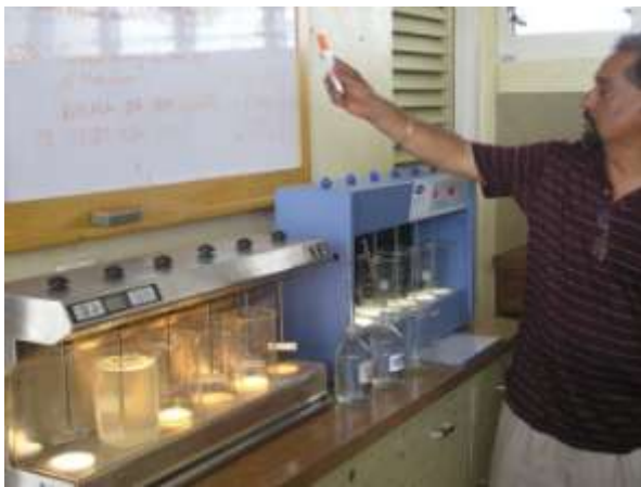
Jar Testing for correct chemical dosing
